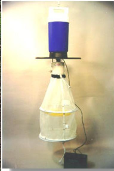
**These are standard dry ice mosquito traps. The thermos-like casing that holds the dry ice is blue with a white lid. A net is attached below the thermos and a battery (shown connected to trap at left) powers a fan and rests on the ground. These traps are generally hung from a tree 4 to 6 feet from the ground (as shown in picture at far left).**
