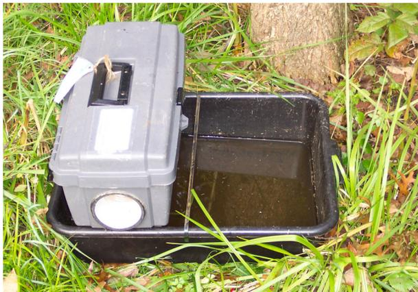
**These traps are gravid traps and use stagnant water as an attractant to lure mosquitoes to a net. They are placed on the ground during the day and are picked up the following morning. A battery is also used to power the fan inside the trap.**
